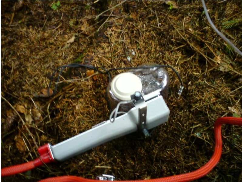
Slika 1. Izgled komore za merenje disanja zemljišta Figure 1. The chamber for soil respiration measurement
