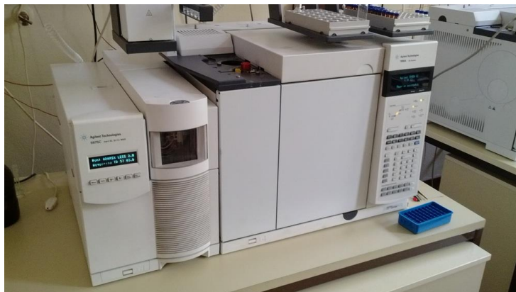
Picture 2. GC-MS Agilent system used for identification of evaporative chemical compounds from poplar leaves (picture taken by the first author, on 16th of August, 2013 in main Centre for Instrumental Analysis laboratory, Faculty for chemistry in Belgrade)
